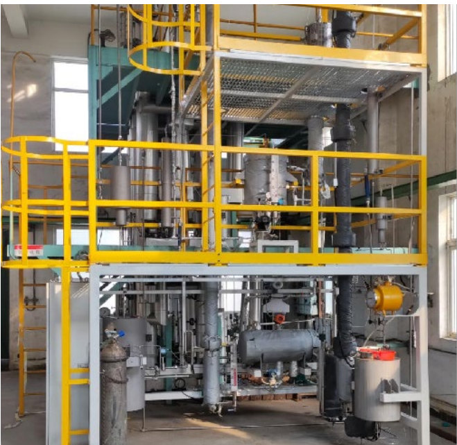
Figure 2: 3Nm 3 /h phase change absorber enlarge test
